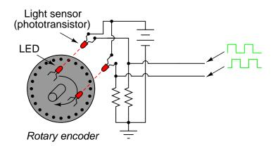
The two LED/phototransistor pairs are arranged in such a way that their pulse outputs are always  $90^{\circ}$  out of phase with each other. Quadrature output encoders are useful because they allow us to determine direction of motion as well as incremental position.
