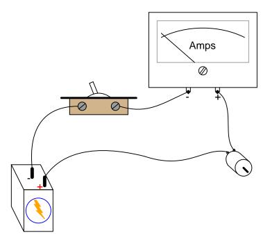
In view of Ohm's Law, where current is supposed to be a direct function of voltage and resistance  $(I = \frac{E}{R})$ , explain why this happens. After all, the motor's winding resistance does not change as it spins, and the battery voltage is fairly constant. Why, then, does the current vary so greatly between initial start-up and full operating speed?
