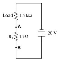
We will have to plot a load line for this simple two-resistor circuit along with the "characteristic curve" for resistor  $R_1$  in order to see the benefit of a load line. Load lines really only have meaning when superimposed with other plots. First, the characteristic curve for  $R_1$ , defined as the voltage/current relationship between terminals **A** and **B**:
