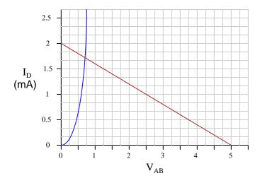
Follow-up question: explain why the use of a load line greatly simplifies the determination of circuit current in such a diode-resistor circuit.
