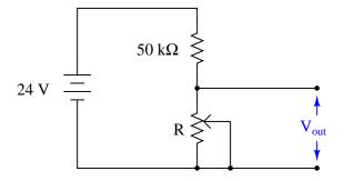
Desired range for  $V_{out} = 0$  to 17 volts
