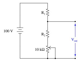
Desired range for  $V_{out} = 30 \text{ volts to } 70 \text{ volts}$
