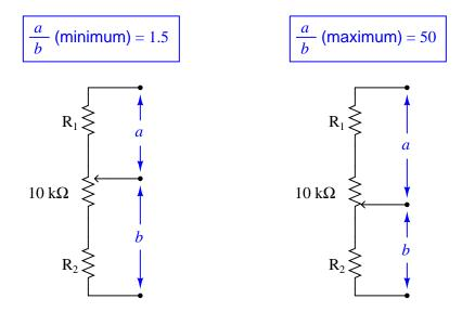
First, write an equation for each circuit, showing how resistances  $R_1$ ,  $R_2$ , and the 10 k $\Omega$  of the potentiometer combine to form the ratio  $\frac{a}{b}$ . Then, use techniques for solving simultaneous equations to calculate actual resistance values for  $R_1$  and  $R_2$ .
