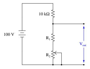
Desired range for  $V_{out} = 30$  volts to 70 volts
