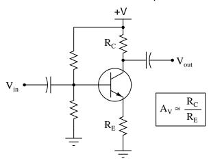
Knowing this, calculate the necessary resistance values for the following fixed-value resistors ( $R_1$  and  $R_2$ ) to give this common-emitter amplifier an adjustable voltage gain range of 4 to 7:
