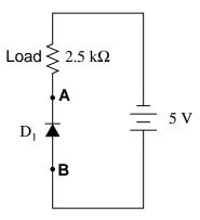
The diode's characteristic curve is already plotted on the following graph. Your task is to plot the load line for the circuit on the same graph, and note where the two lines intersect:
