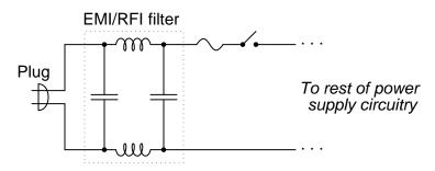
Determine what type of filter circuit this is (LP, HP, BP, or BS), and also determine the inductive and capacitive reactances of its components at 60 Hz, if the inductors are 100  $\mu$ H each and the capacitors are 0.022  $\mu$ F each.
