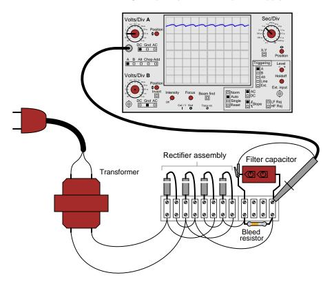
The waveform shown by the oscilloscope is mostly DC, with just a little bit of AC "ripple" voltage appearing as a ripple pattern on what would otherwise be a straight, horizontal line. This is quite normal for the output of an AC-DC power supply.
