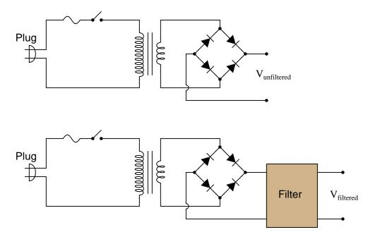
Draw the respective output voltage waveforms of these two power supply circuits ( $V_{unfiltered}$  versus  $V_{filtered}$ ). Also identify the type of filter circuit needed for the task (low pass, high pass, band pass, or band stop), and explain why that type of filter circuit is needed. file 00789
