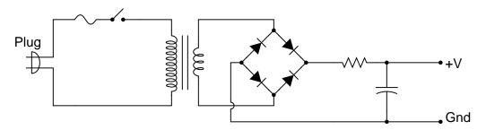
While this design will work, there are better filter configurations for this application. Describe the limitations of the circuit shown, and explain how some of the other filters would do a better job.
