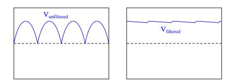
A low pass filter is the kind needed to filter "ripple voltage" from the power supply output.
