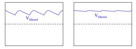
If both of these waveforms were measured on the same power supply circuit, at different times, determine which waveform was measured during a period of heavier "loading" (a "heavier" load being defined as a load drawing *greater* current).
