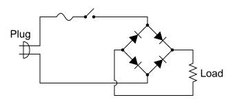
However, this form of AC-to-DC power conversion has some significant limits. Explain why most power supply circuits utilize a transformer instead of directly rectifying the line power as this circuit does. file 02016
