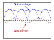
The non-filtered DC output waveform is still shown as a dotted line, for reference purposes.  $\underline{file~00793}$
