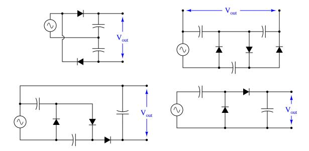
Determine the degree of voltage multiplication (double, triple, etc.) provided by each circuit.  $\underline{file\ 02011}$
