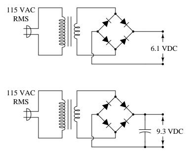
Explain why this is. How can the addition of nothing but a capacitor have such a great effect on the amount of DC voltage output by the circuit?
