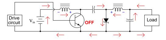
Follow-up question: how does the load voltage of this converter relate to the supply (battery) voltage? Does the load receive more or less voltage than that provided by the battery?
