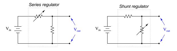
Typically, these variable resistances are provided by transistors rather than actual rheostats, which would have to be manually controlled.
