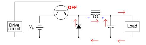
Follow-up question: how does the load voltage of this converter relate to the supply (battery) voltage? Does the load receive more or less voltage than that provided by the battery?
