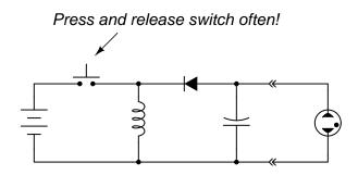
Follow-up question: how would you recommend we "automate" this circuit so that a person does not have to keep pressing and releasing the switch for it to generate a continuous DC output voltage?
