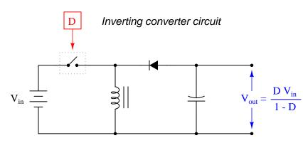
Based on this mathematical relationship, calculate the output voltage of this converter circuit at these duty cycles, assuming an input voltage of 40 volts:
