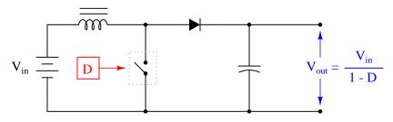
Based on this mathematical relationship, calculate the output voltage of this converter circuit at these duty cycles, assuming an input voltage of 40 volts:
