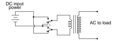
The first commercially available inverters produced simple square-wave output:
