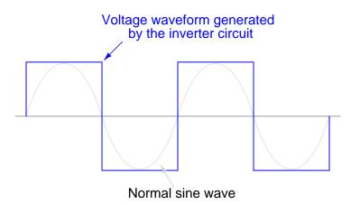
However, this caused problems for most power transformers designed to operate on sine-wave AC power. When powered by the square-wave output of such an inverter, most transformers would *saturate* due to excessive magnetic flux accumulating in the core at certain points of the waveform's cycle. To describe this in the simplest terms, a square wave possesses a greater *volt-second product* than a sine wave with the same peak amplitude and fundamental frequency.
