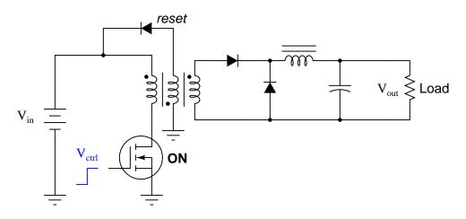
Now, trace current through the circuit while the transistor is off, and explain the purpose of the *reset* winding in the transformer:
