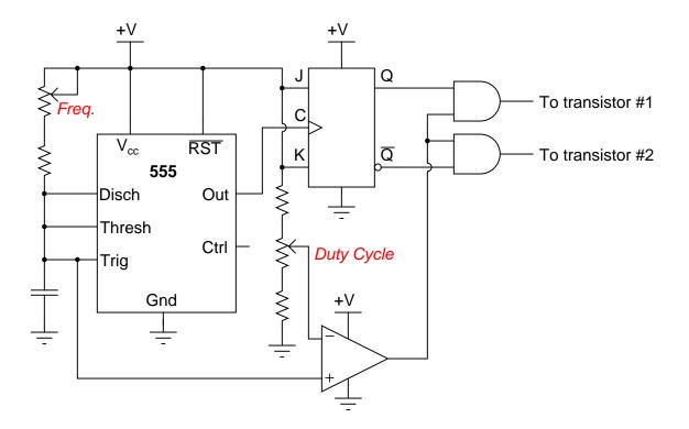
Follow-up question: which direction would you have to move the frequency potentiometer to increase the output frequency of this circuit? Which direction would you have to move the duty cycle potentiometer to increase that as well?
