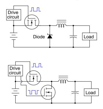
The diode is a simple solution for providing the inductor a path for current when the main switching transistor is off. Why would anyone use another MOSFET in place of it, especially if this means the drive circuit has to become more complex (to drive two transistors at different times instead of just one transistor) to do the same task?
