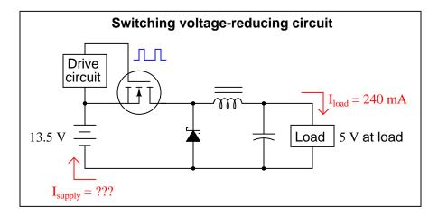
Calculate the average supply current  $(I_{supply})$  for both of these circuits. Assume that the switching circuit has negligible power losses in the transistor, inductor, capacitor, and diode. If the 13.5 volt source were an electrochemical battery, which battery would last longer powering the same load? <u>file 02479</u>
