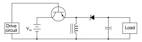
In this circuit, the transistor is either fully on or fully off; that is, driven between the extremes of saturation or cutoff. By avoiding the transistor's "active" mode (where it would drop substantial voltage while conducting current), very low transistor power dissipations can be achieved. With little power wasted in the form of heat, "switching" power conversion circuits are typically very efficient.
