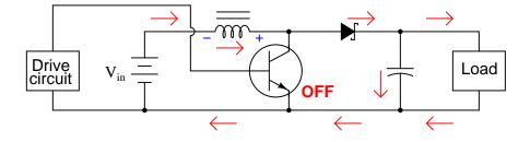
Follow-up question: how does the load voltage of this converter relate to the supply (battery) voltage? Does the load receive more or less voltage than that provided by the battery?
