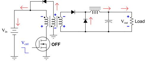
The purpose of the reset winding is to rid the transformer core of stored energy during the off cycle. If this were not done, the transformer core's magnetic flux levels would reach saturation after just a few on/off cycles of the transistor.
