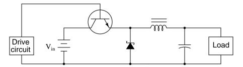
In this circuit, the transistor is either fully on or fully off; that is, driven between the extremes of saturation or cutoff. By avoiding the transistor's "active" mode (where it would drop substantial voltage while conducting current), very low transistor power dissipations can be achieved. With little power wasted in the form of heat, "switching" power conversion circuits are typically very efficient.
