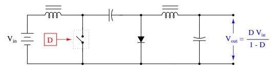
Based on this mathematical relationship, calculate the output voltage of this converter circuit at these duty cycles, assuming an input voltage of 25 volts:
