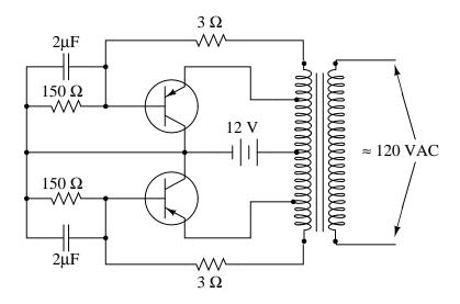
The 120 volt AC output provided by this circuit is definitely *not* sinusoidal, and the circuit's frequency varies with load. Can you think of any way(s) to improve these aspects of the circuit (you need not show details of your design modifications)?
