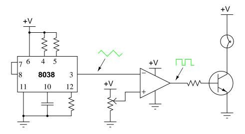
The result is a pulse waveform to the base of the power transistor, of the same frequency as the sawtooth waveform. Normally in circuits such as this, the frequency is at least several hundred Hertz.
