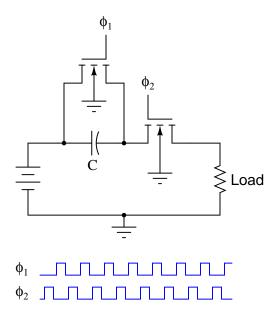
Note: the  $\phi_1$  and  $\phi_2$  pulse signals are collectively referred to as a non-overlapping, two-phase clock.
