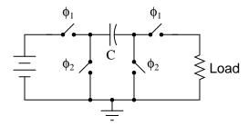
Identify the polarity of voltage across the load resistor in the following switched capacitor circuit. Note: the only difference between this circuit and the last is the switching sequence.
