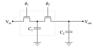
$$f_{-3dB} = \frac{f_{switch}C_1}{2\pi C_2}$$
