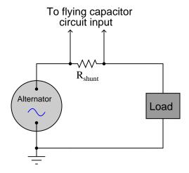
The frequency of the alternator's output is 50 Hz. How does this affect the design of the flying capacitor circuit, so we ensure a fairly accurate reproduction of the AC signal at the output of the flying capacitor circuit? Generalize your answer to cover all conditions where the input signal varies over time.
