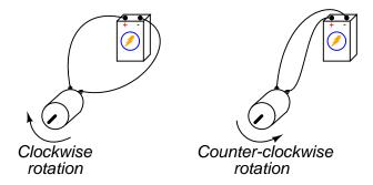
Complete this schematic diagram, showing how a DPDT switch may be placed in this circuit to reverse the motor's direction of rotation without the need to disconnect and re-connect wires:
