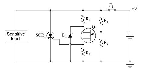
Here, the UJT serves as an overvoltage detection device, triggering the SCR when necessary. Explain how this circuit works, and what the function of each of its components is. file 02143
