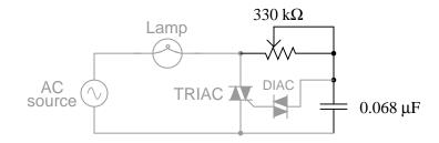
Calculate how many degrees of phase shift the capacitor's voltage is, compared to the total voltage across the series RC network, assuming a frequency of 60 Hz, and a 50% potentiometer setting. <u>file 00637</u>
