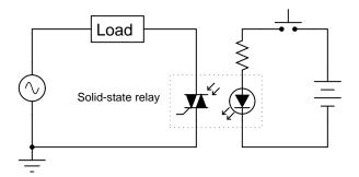
Describe some of the advantages of using a solid-state relay for switching AC power instead of using an electromechanical relay as shown here:
