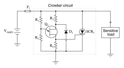
Measuring the supply voltage with a voltmeter, everything checks out well. There does not appear to be an overvoltage condition causing a legitimate "crowbar" event in the circuit. Disconnecting the load from the crowbar circuit and powering it up with a standard bench-top laboratory power supply reveals the load to be in perfect condition. Thus, both the source and the load have been eliminated as possibilities that may have blown the fuse(s).
