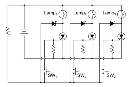
Explain how this circuit works. Why can't any of the other lamps turn on once any one of them has been energized? Also, explain how the circuit could be modified so as to provide a "reset" to turn all lamps off again.
