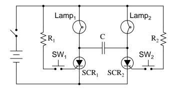
When the power is first turned on, neither lamp will energize. If either pushbutton switch is then momentarily actuated, the lamp controlled by that SCR will energize. If, after one of the lamps has been energized, the *other* pushbutton switch is then actuated, its lamp will energize *and the other lamp will de-energize*.
