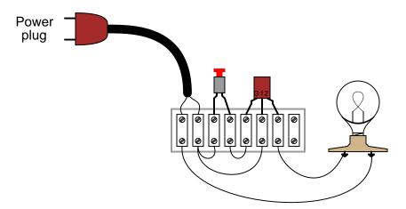
When the pushbutton switch is actuated, nothing happens. What is wrong with this circuit? Hint: the problem in this circuit is very subtle, and may be very difficult to discern. file 01091
