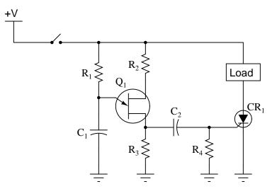
Together, the combination of  $R_1$ ,  $C_1$ ,  $R_2$ ,  $R_3$ , and  $Q_1$  form a *relaxation oscillator*, which outputs a square wave signal. Explain how a square wave oscillation is able to perform a simple time-delay for the load, where the load energizes a certain time *after* the toggle switch is closed. Also explain the purpose of the RC network formed by  $C_2$  and  $R_4$ .
