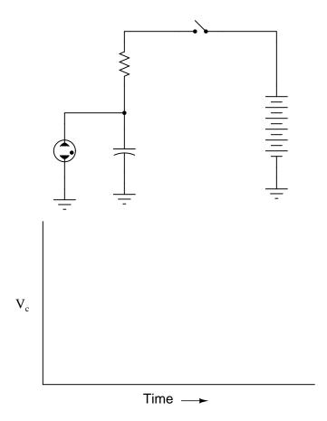
Graph the capacitor's voltage over time as this circuit is energized by the DC source. Note on your graph at what times the neon bulb is lit:
