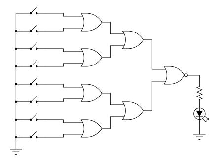
As is common in digital circuit schematics, the power supply  $(V_{CC})$  is omitted for the sake of simplicity. This is analogous to the omission of power supply connections in many operational amplifier circuit schematics.
