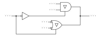
What, specifically, causes gates to be damaged by "paralleling" their outputs? Generally speaking, what principle must be followed in order to "parallel" logic gate outputs without risk of damage? Explain how each of the three acceptable "paralleled" scenarios shown here meet this criterion.
