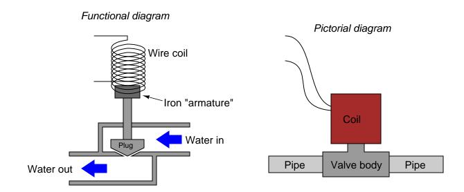
Some solenoid valves are constructed in such a way that the coil assembly may be removed from the valve body, separating these two pieces so that maintenance work may be done on one without interfering with the other. Of course, this means the valve mechanism will no longer be actuated by the magnetic field, but at least one piece may be worked upon without having to remove the other piece from whatever it may be connected to:
