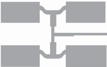
Figure 6.17 Geometry of  $2 \times 2$  sub-array.
