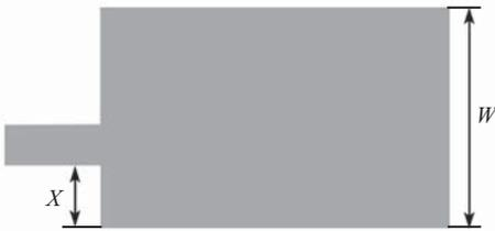
Figure 5.31 Microstrip patch antenna.
